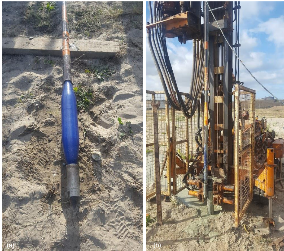
Figure 3.7 – (a) Photo of the probe assembled for the tests at Dunkirk site; (b) photo taken before probe insertion into the ground
