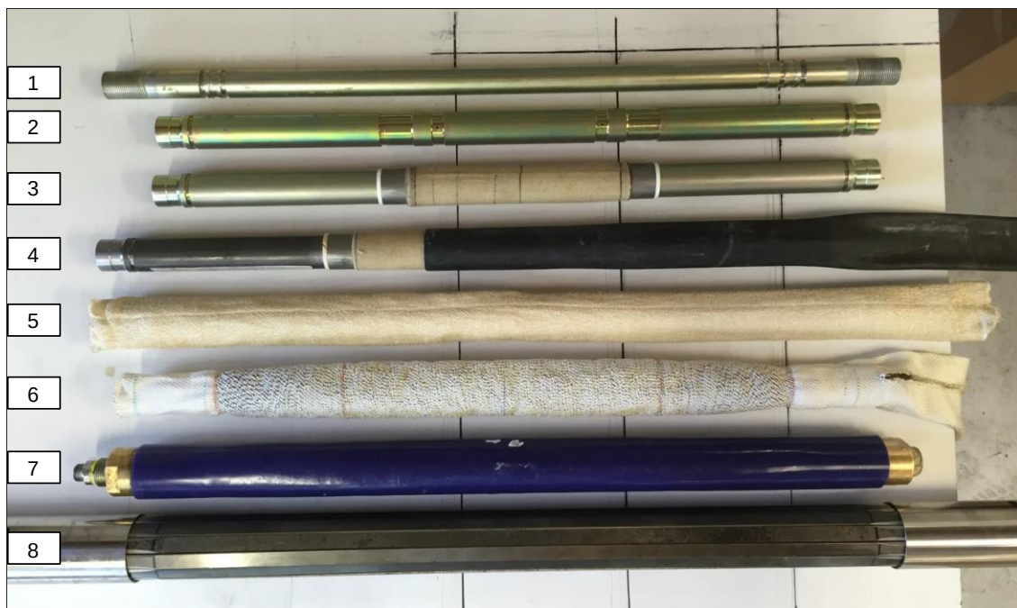
Figure A.18 – Component layers of a FC 60 probe (adapted from Cour and Rouet (2017))
