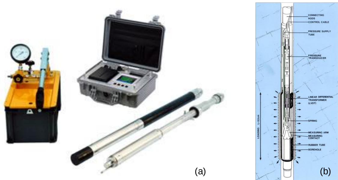
Figure A.14 – (a) OYO Elastmeter monocell pressuremeter probe for high-pressure applications (up to 20 MPa). Radial displacement transducers used to assess radial strain. (b) Probe scheme showing the displacement transducers OYO (2019c), (2019d)
