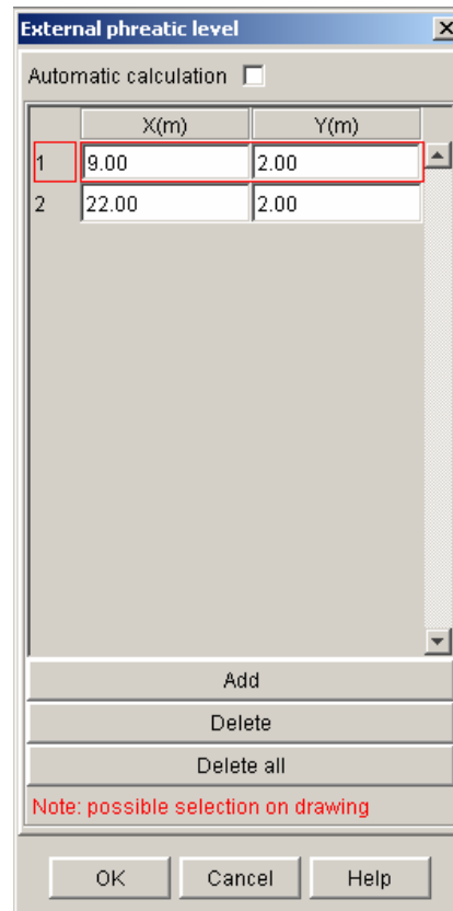
Figure 75: definition of the external phreatic line for stage 2
