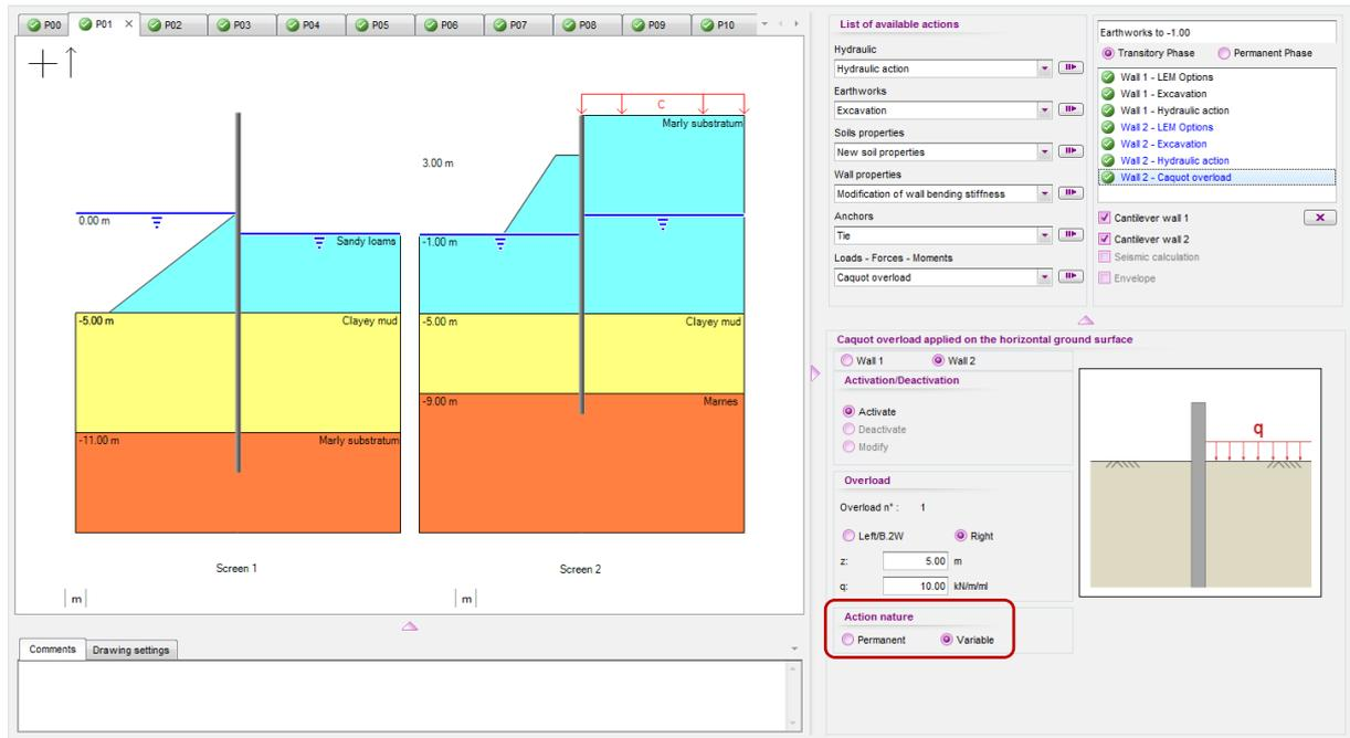
The screenshot displays two soil profiles, Screen 1 and Screen 2. Screen 1 shows layers of Marly substratum (0 to -11.00 m), Clayey mud (-11.00 to -5.00 m), and Sandy loams (-5.00 to 0.00 m). Screen 2 shows layers of Marles (0 to -9.00 m), Clayey mud (-9.00 to -5.00 m), and Sandy loams (-5.00 to 3.00 m). The 'List of available actions' panel on the right shows 'Caquot overload' selected under 'Loads - Forces - Moments'. The 'Action nature' is set to 'Variable'.
