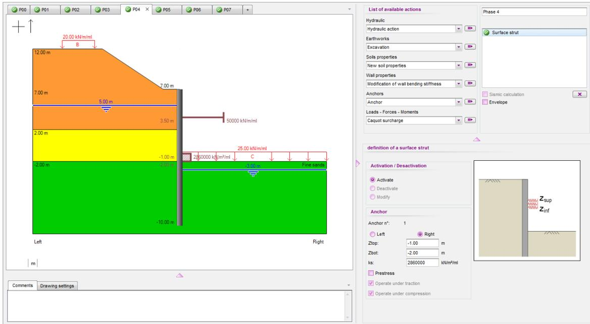
D.2.1.4.6. Phase 5: Removal of the layer of struts + construction of cover slab
