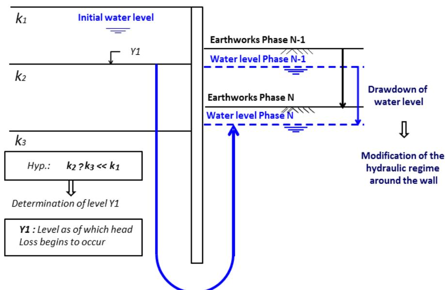
The following figure illustrates the flow field which develops in the soil in the case of a homogeneous soil. This is characterised by:
