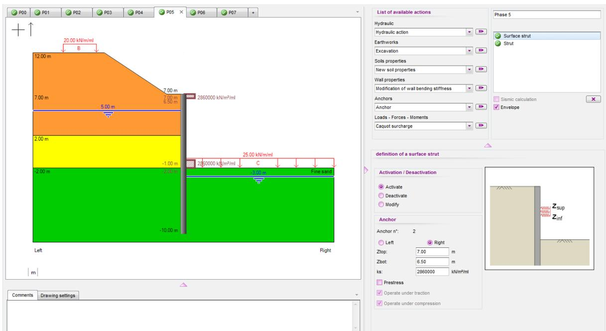
D.2.1.4.7. Phase 6: Start-up of the structure and stop of the pumping
