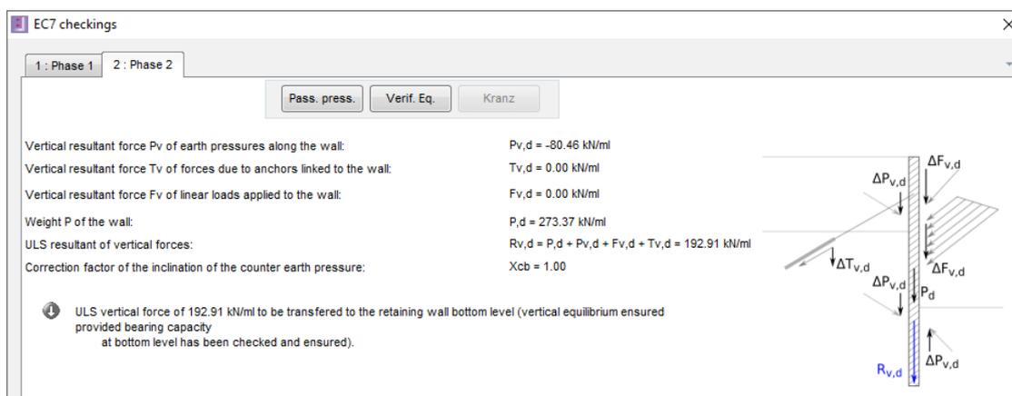
The above window also shows a factor  $X_{cb}$ , known as the “Correction factor of the inclination of the counter earth pressure” the meaning of which will be detailed in the next chapter.
