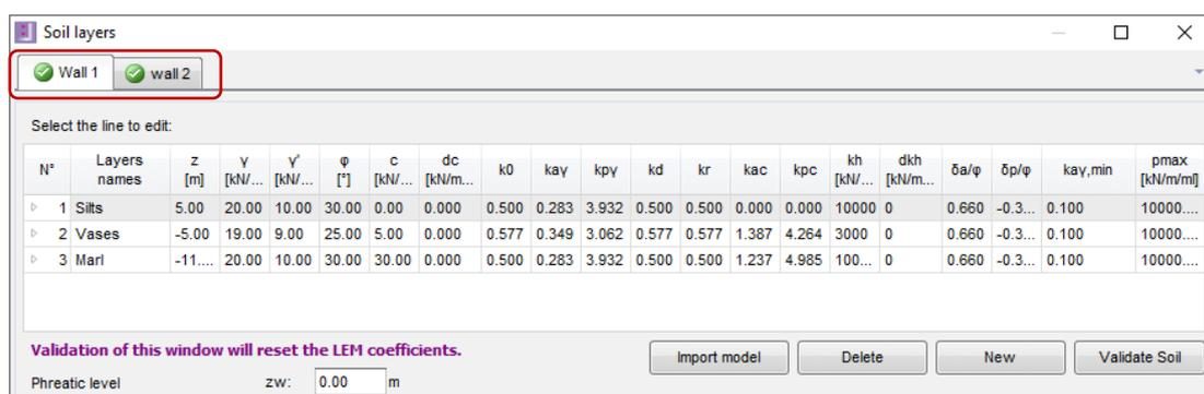
It is possible to import into wall 2 the parameters already filled out for wall 1 by going to the "Wall 2" tab and clicking **Import model**. Then modify the level of the top of the Marl to -9.00 for wall 2.
