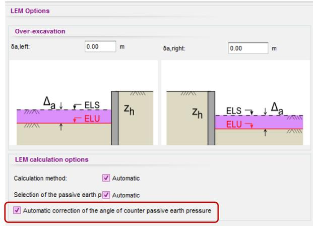
This option allows automatic readjustment of the counter passive earth pressure angles if the vertical equilibrium verification leads to an upwards resultant. The counter earth pressure angle considered in the calculation is as follows:
