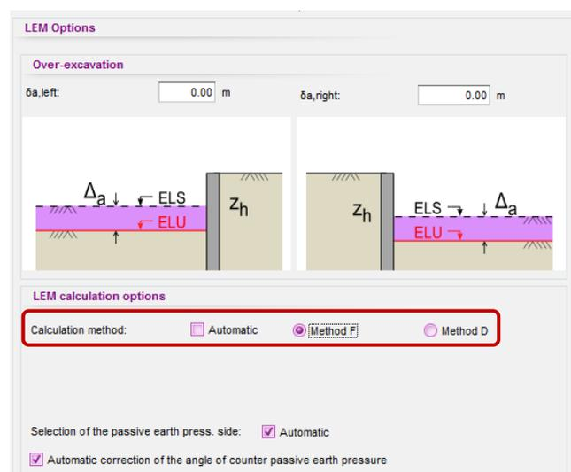
Start the calculation and compare the results obtained (moment diagrams, details of ULS checks) with those of a LEM-D calculation. The following table summarises this comparison.
