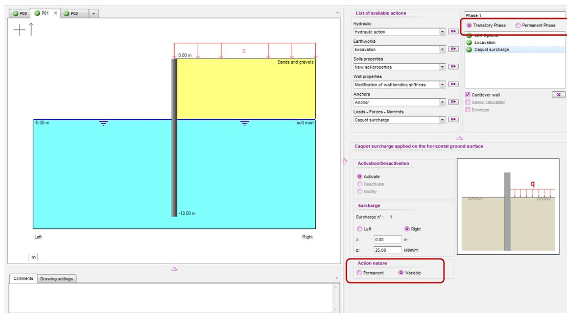
This project (and thus this phase) includes no anchors and the wall is cantilever. Moreover, we activated the ULS checks when defining the properties of the project.
