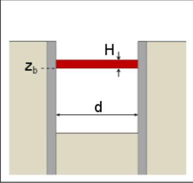
Linking anchors are the only interactions taken into account between the two walls. There is no interaction considered between the two walls through the soil.
