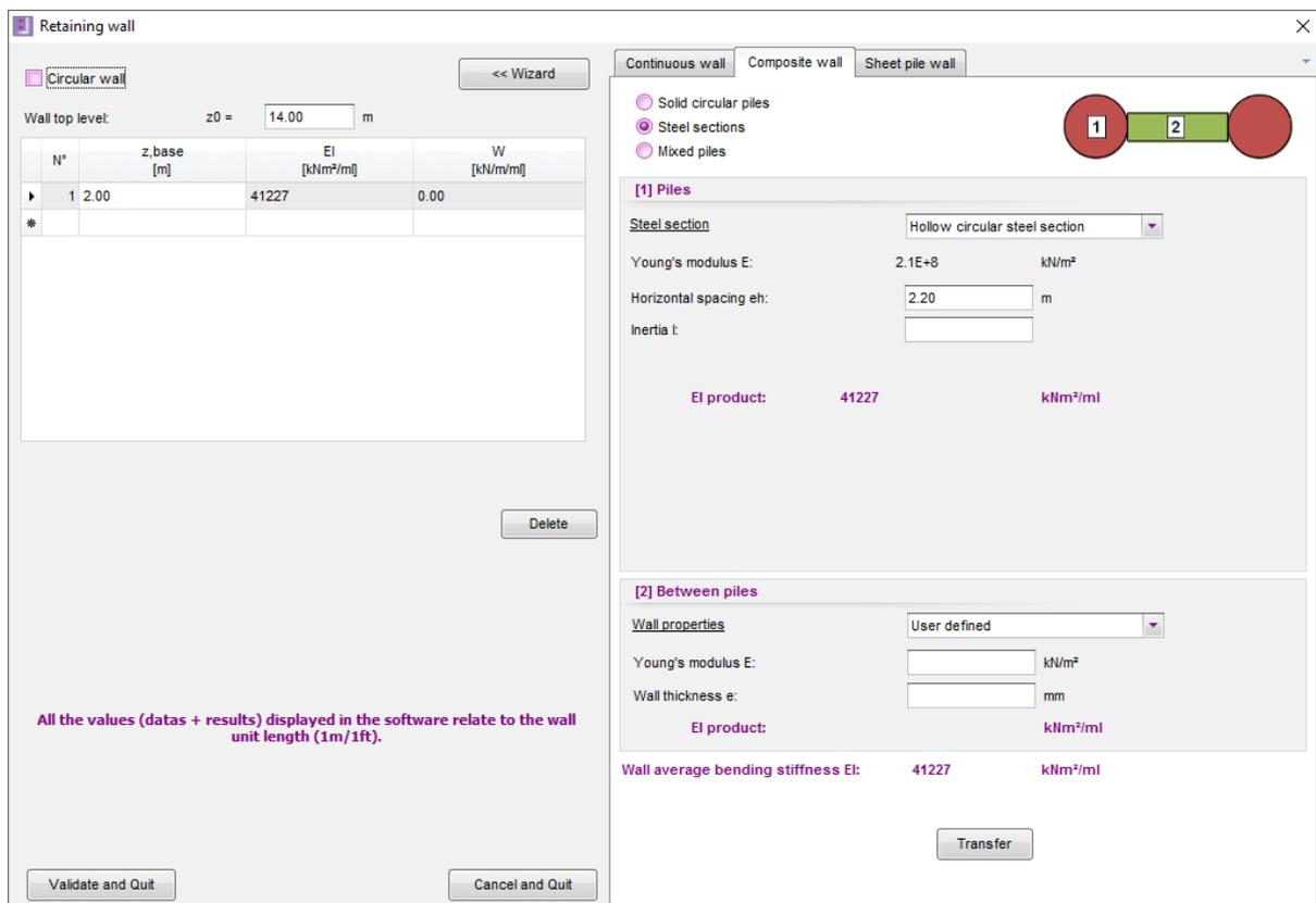
Finally, click  to take account of the values input and the data will appear on the graphic representation of the project initial data. To modify the characteristics of the wall subsequently, click the **Data** menu, then **Wall Definition**.
