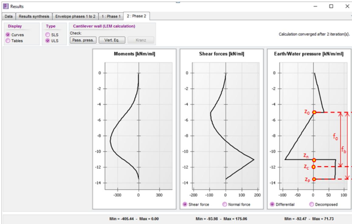
The following figure provides the details of the check of the passive earth pressures for this phase. In the present case, we have  $f_b = 1.22 f_0$ . The wall embedment depth is thus optimum for the passive earth pressure safety check.
