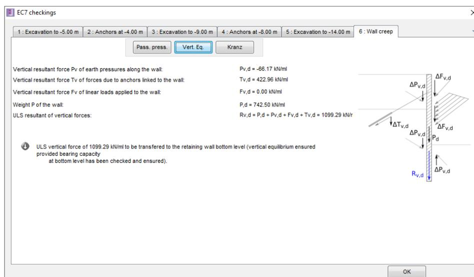
Here, for phase 6, the vertical resultant of the forces is evaluated (at ULS) at about 1 100 kN/ml, which corresponds to a base resistance of  $1\ 100 / 1.0 = 1.1 \text{ Mpa}$ , which is acceptable given the nature of the supporting soil (Marls with  $p_l > 3 \text{ MPa}$ ).
