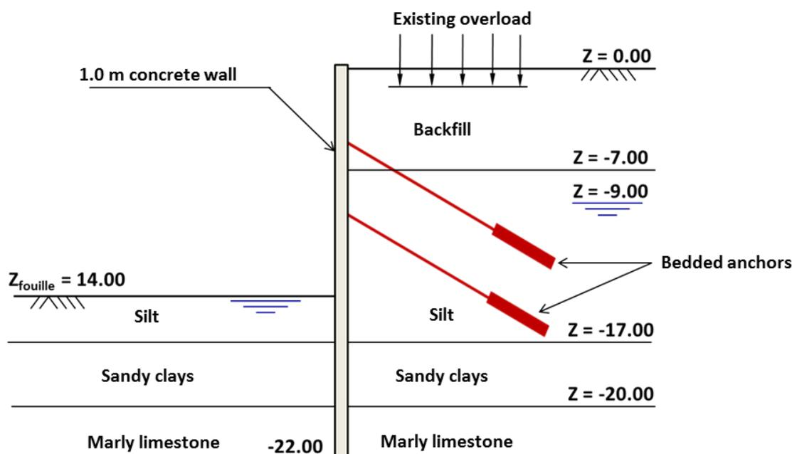
This example mainly aims to demonstrate the K-Réa functionalities linked to the ULS checks according to EC7, more specifically with regard to the stability of the anchor block in the case of a wall anchored by one or more layers of bedded anchors.
