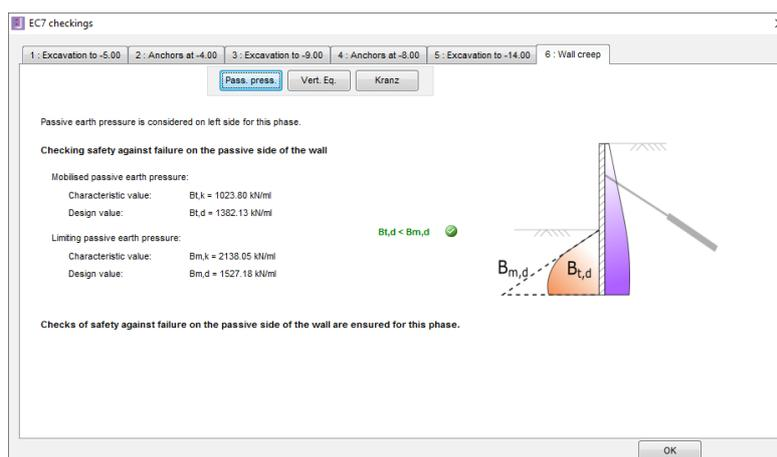
Application of a "1.40" factor to the mobilisable passive earth pressure can be explained by the fact that phase 6 (just like phase 5) is considered to be "permanent".
