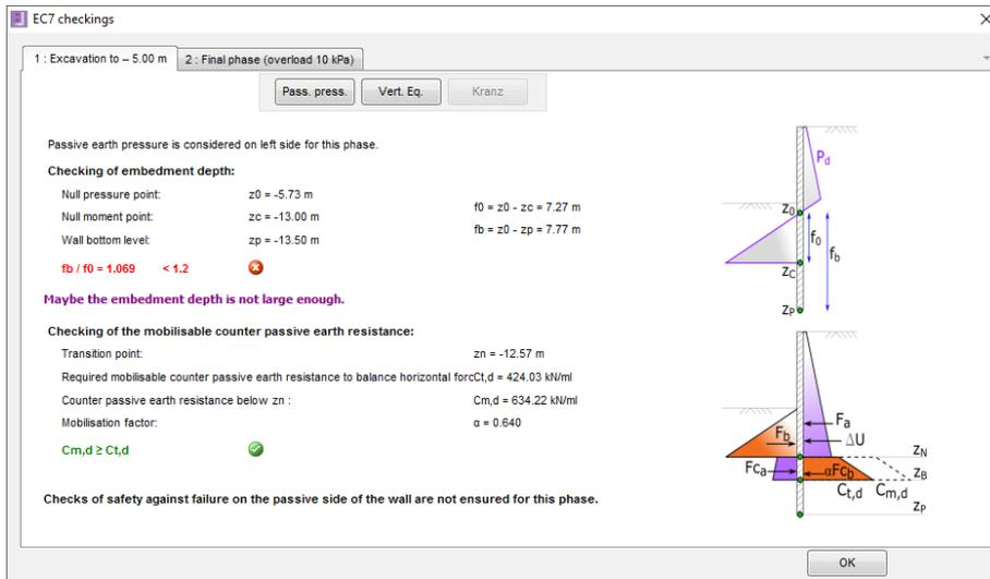
The search for the optimum embedment depth shows that the verification of the passive earth pressure safety check taking account of an over-excavation of 0.5 m requires extension of the wall by 1.50 m by comparison with the length initially validated in the absence of over-excavation. The result obtained with a wall base at -15.00 is presented below.
