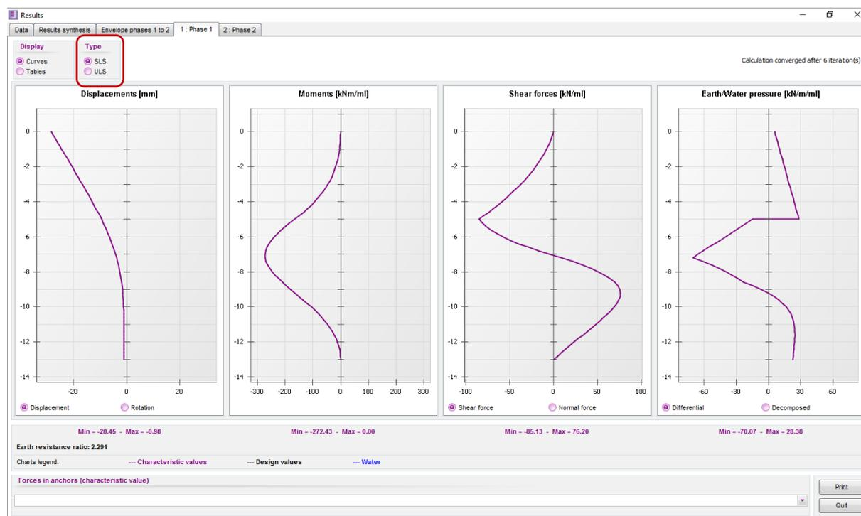
The following figure presents the ULS results of phase 1: only the moments, shear forces and pressures diagrams are available (no displacements with the LEM model). The forces and pressures are expressed directly in calculation values (ULS). The maximum values are as follows:
