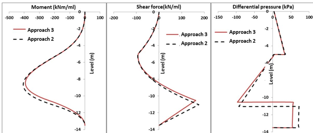
However, approach 3 is unable to differentiate the transitory phases from the permanent phases (approach 2 considers a smaller safety margin on the passive earth pressure in the case of a transitory phase). The comparison with approach 2 in phase 1 (transitory) therefore gives diverging results. Approach 3 leads to more unfavourable results.
