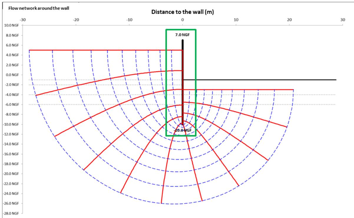
By comparison with the hydrostatic regime in which all the points (on the same side of the wall) are associated with the same hydraulic head (corresponding to the top of the water table on the side concerned), the development of the flow regime leads to a hydraulic head that varies with depth on each side of the wall.
