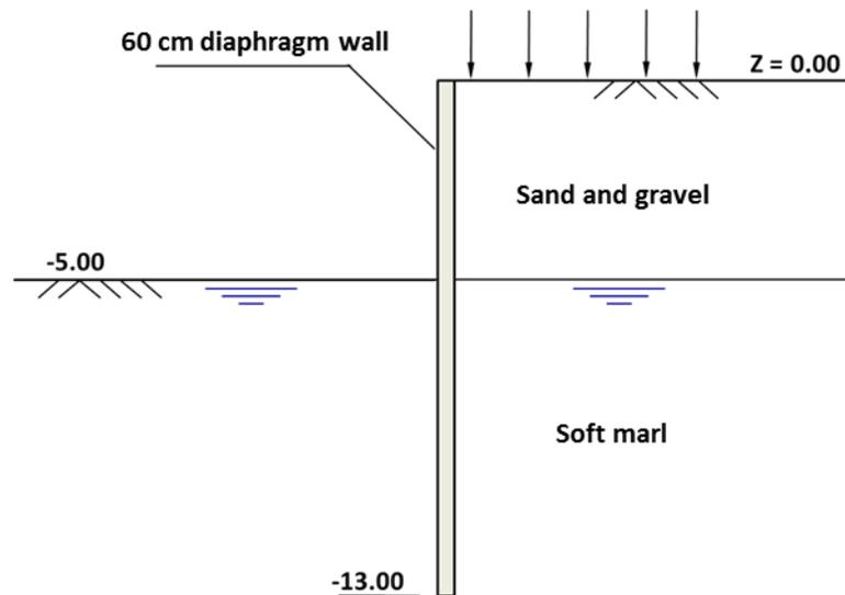
In this example, we will detail the ULS checks for this type of configuration.
