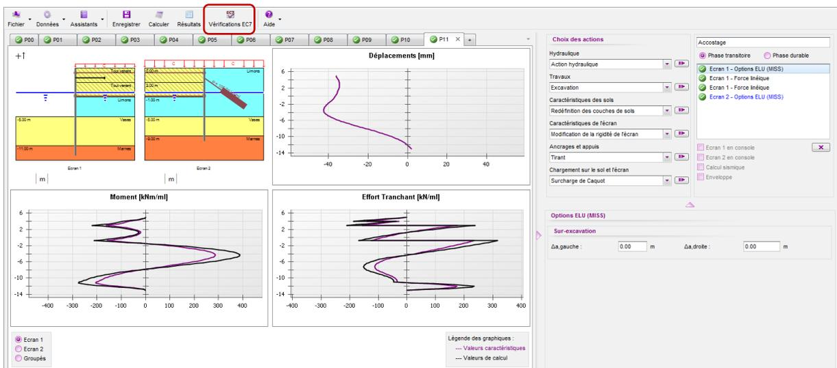
The screenshot shows the 'Vérifications EC7' window with three graphs: 'Déplacements [mm]', 'Moment [kNm/m]', and 'Effort Tranchant [kN/m]'. The 'Options ELU (MSS)' panel on the right shows 'Phase transitoire' selected. The 'Sur-excavation' section shows 'Δa.gauche' and 'Δa.droite' both set to 0.00 m.
