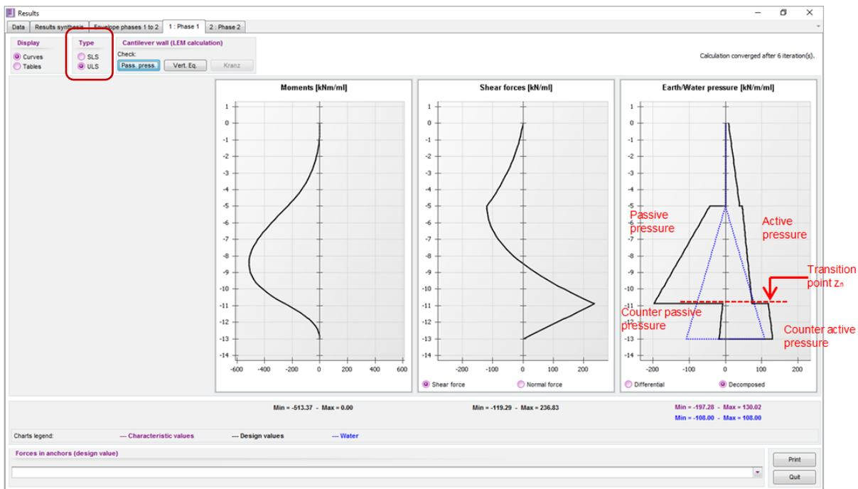
In this phase, the passive earth pressure side was automatically chosen by K-Réa as being the left side. This automatic choice may be forced by the user in the “LEM options” action accessible for each phase in which the wall is declared as cantilever.
