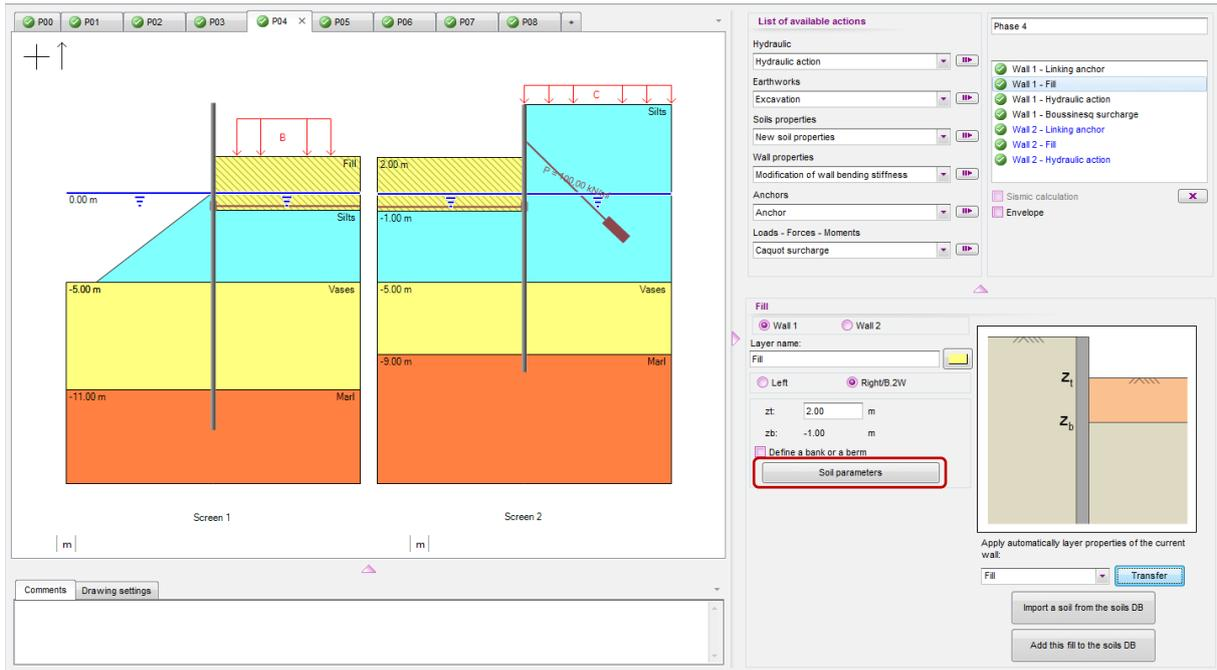
The backfill characteristics are to be filled out in the window accessible via the
