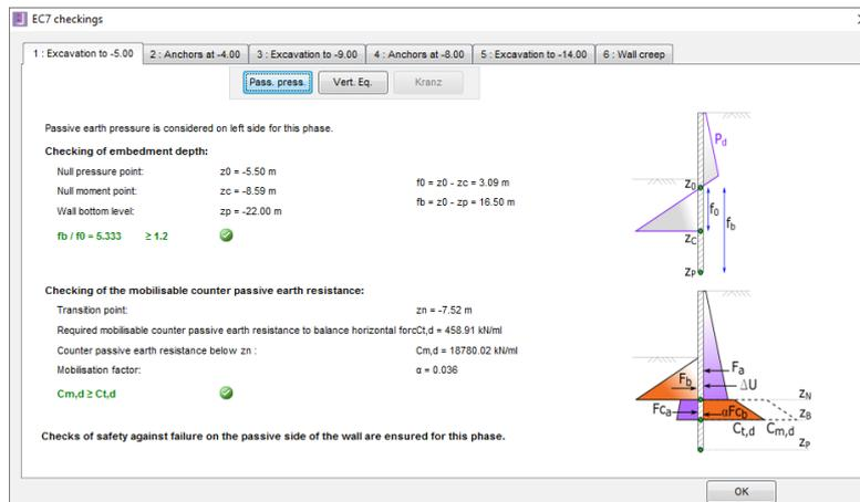
For the following phases (2 to 6), the wall is considered to be “anchored” and therefore the passive earth pressure safety check is based on the MISS calculation. It consists in checking that the mobilisable (or limit) passive earth pressure is greater than the mobilised passive earth pressure, with a sufficient safety margin. For example, for phase 6:
