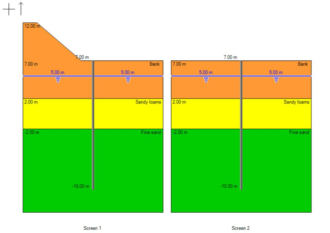
**Phase 1:** elimination of the Boussinesq overload behind the right-hand diaphragm wall (Wall 2)
