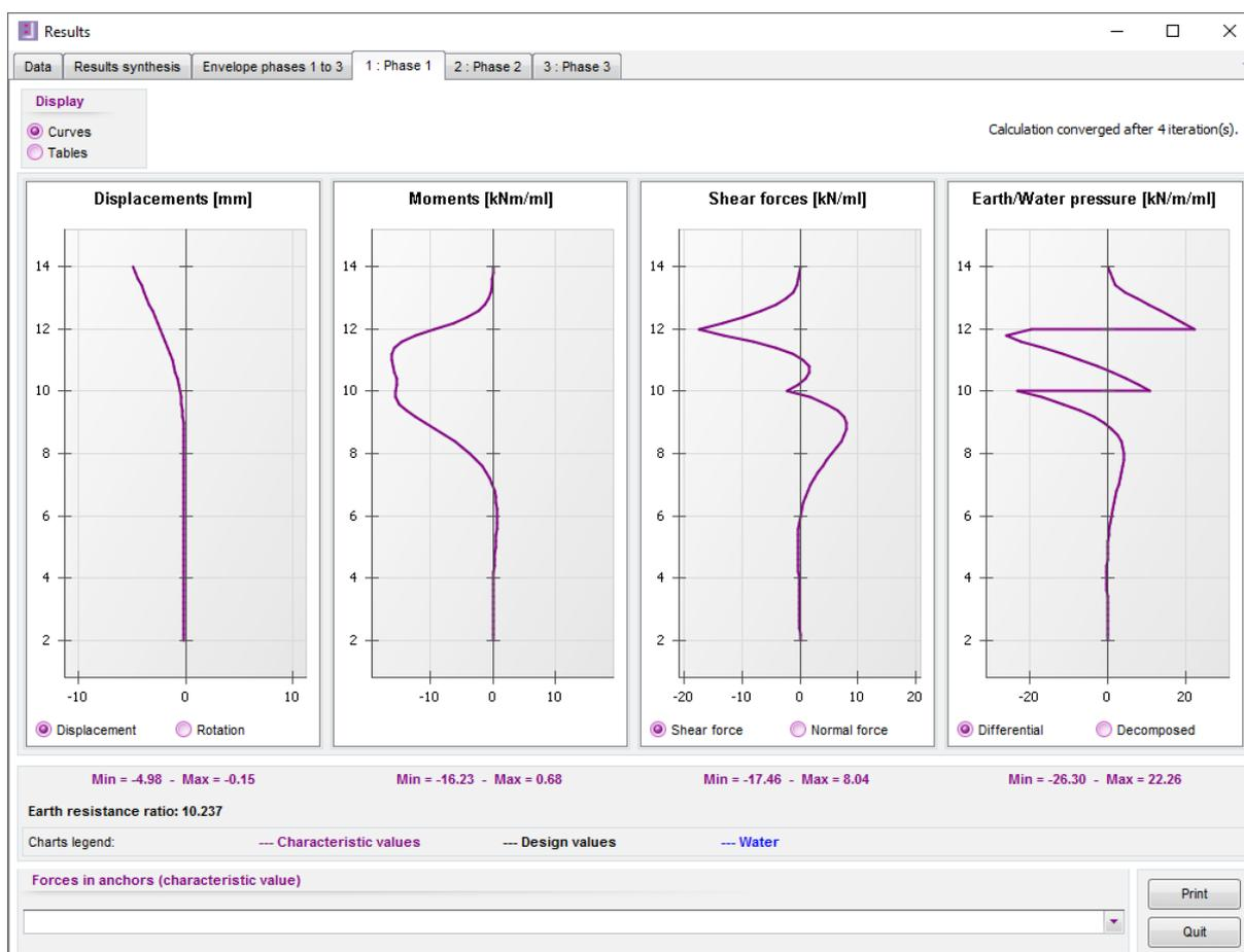
The shape of the curve clearly corresponds to the behaviour of a cantilever wall.
