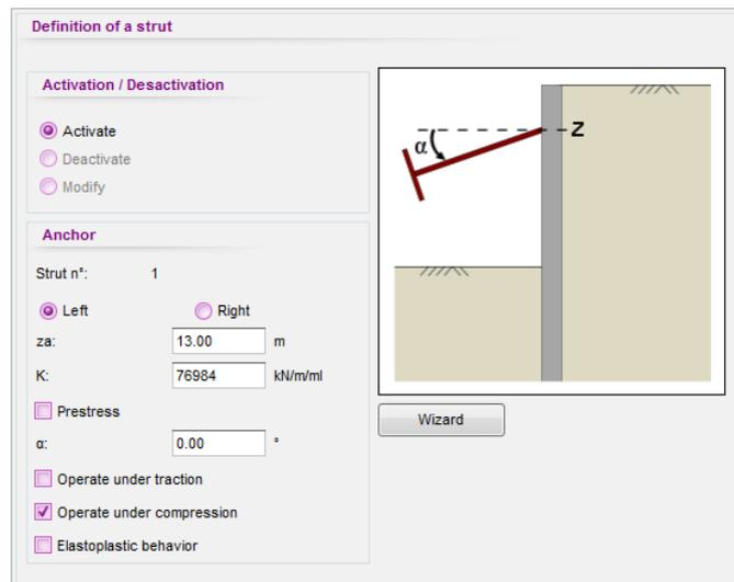
The second action of the 2<sup>nd</sup> phase is excavation with installation of sheeting. To model this, two actions must be used: the **Excavation** action followed by the **Sheeting installation** action:
