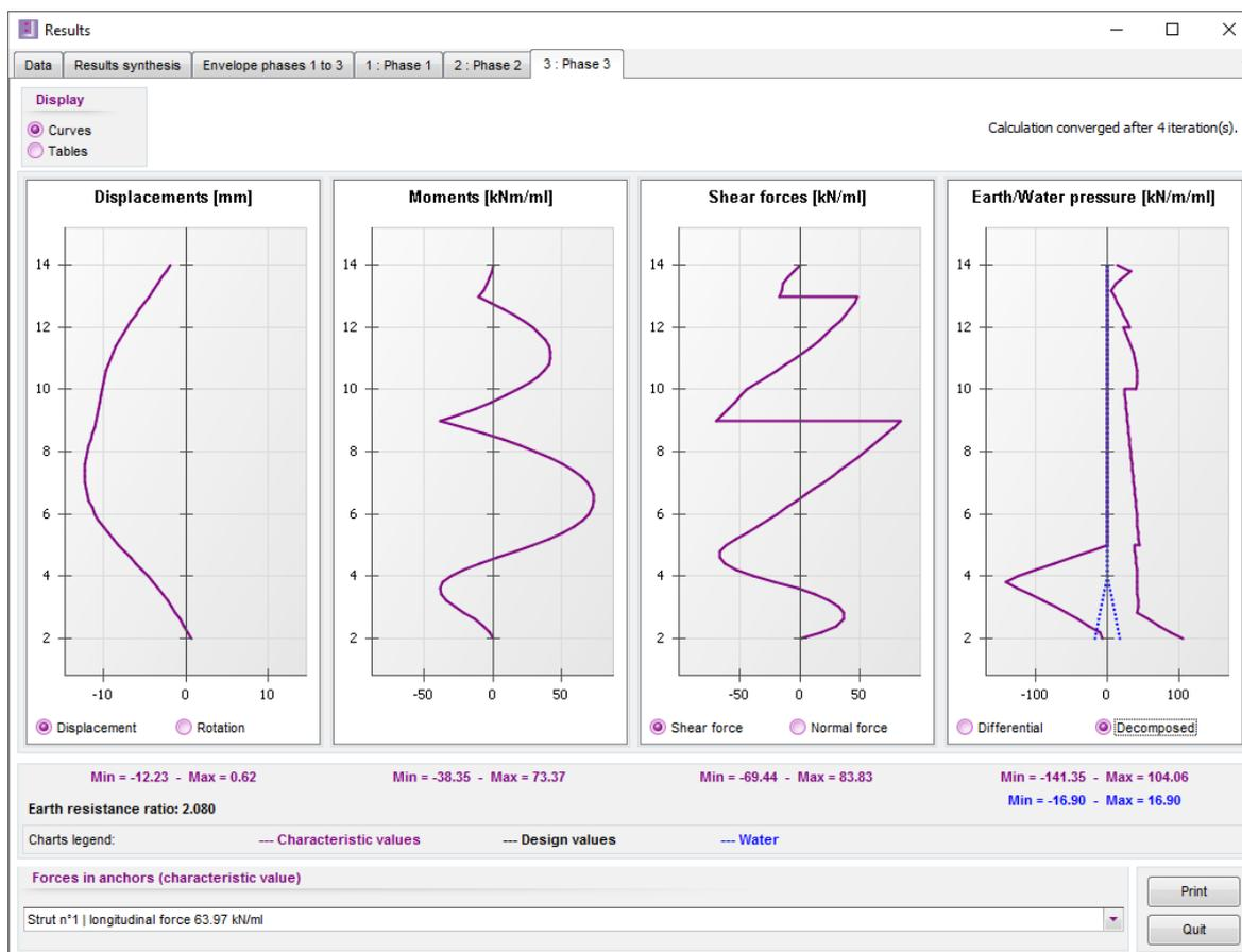
The maximum displacement obtained in phase 3 is about 1 cm.
