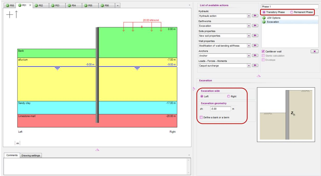
The “Cantilever wall” box is automatically ticked: the ULS equilibrium of the wall will thus be checked by a “LEM” model in this phase.
