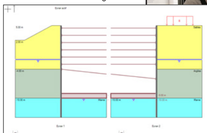
K-Réa v4 – Double-wall project Unlimited number of linking anchors.
